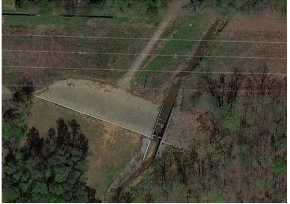
Figure 12: Example of Slot Dam Configuration from Mark Avenue Project in Cobb County
